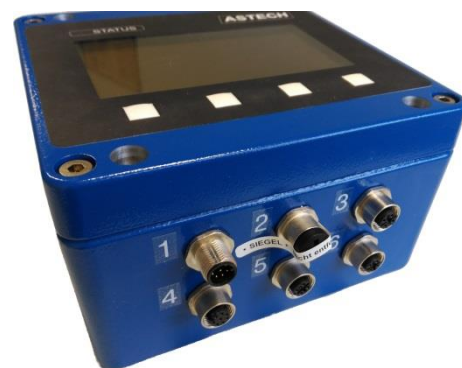
Figure 6: CDB with sealed programming connector
