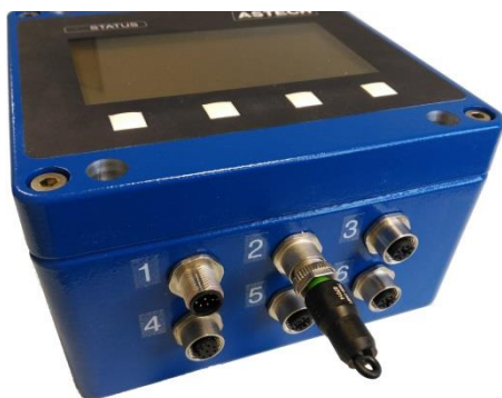
Figure 5: CDB with programming adapter
